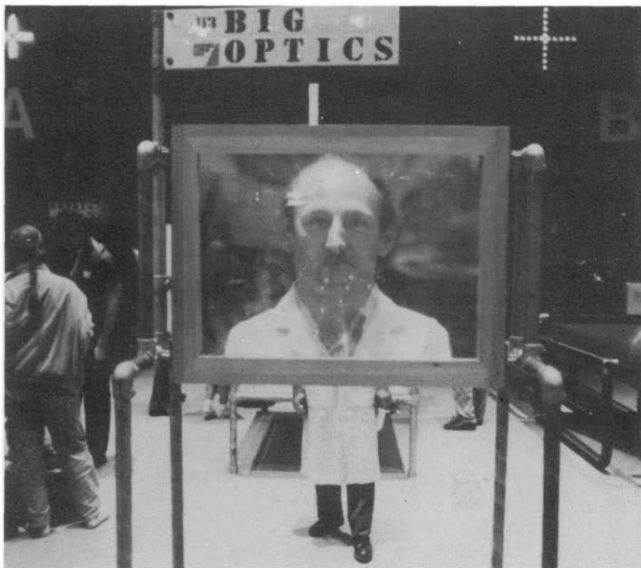
Big Optics. Most people expect magnifying glasses to be curved but this one is flat and made up of wedge shape rings. Great for photographs of your friends.
