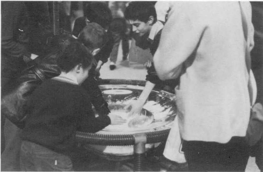
The Salt Bowl. Salt which is packed solid acts as if it were a fluid when air is blown through it.
