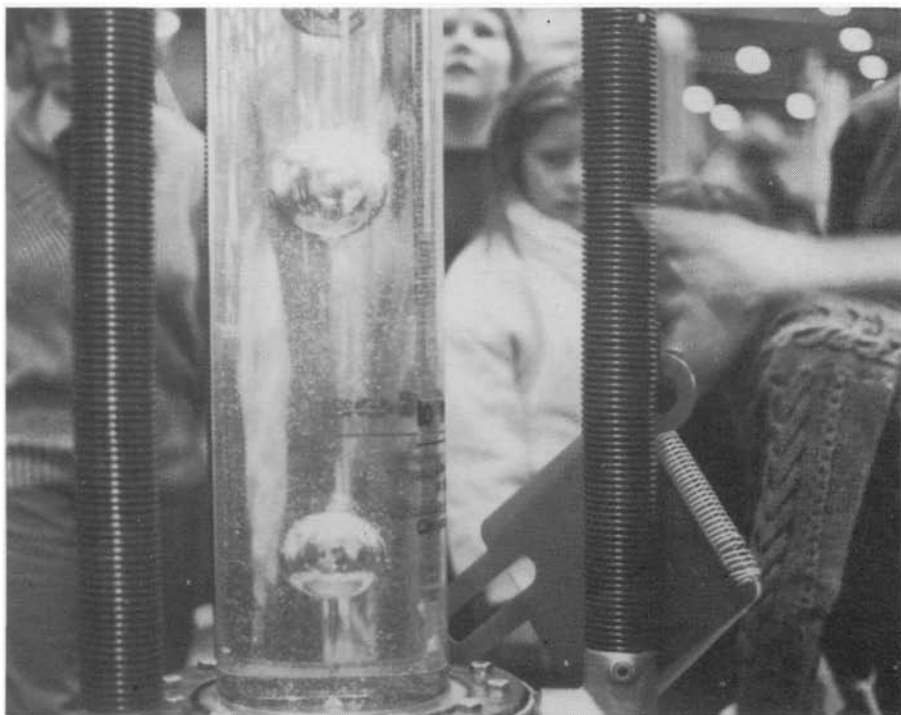
Air bubbles pumped into viscous silicone fluid rise at different rates depending on size. Finding or making a hand pump robust enough proved to be a problem.
